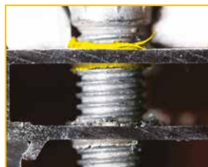
The profile is compressed against the hole of the hinge, forming a collar that eliminates any screw/hinge/profile plays.
